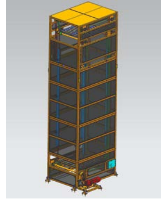
Continuous Pallet Lift
