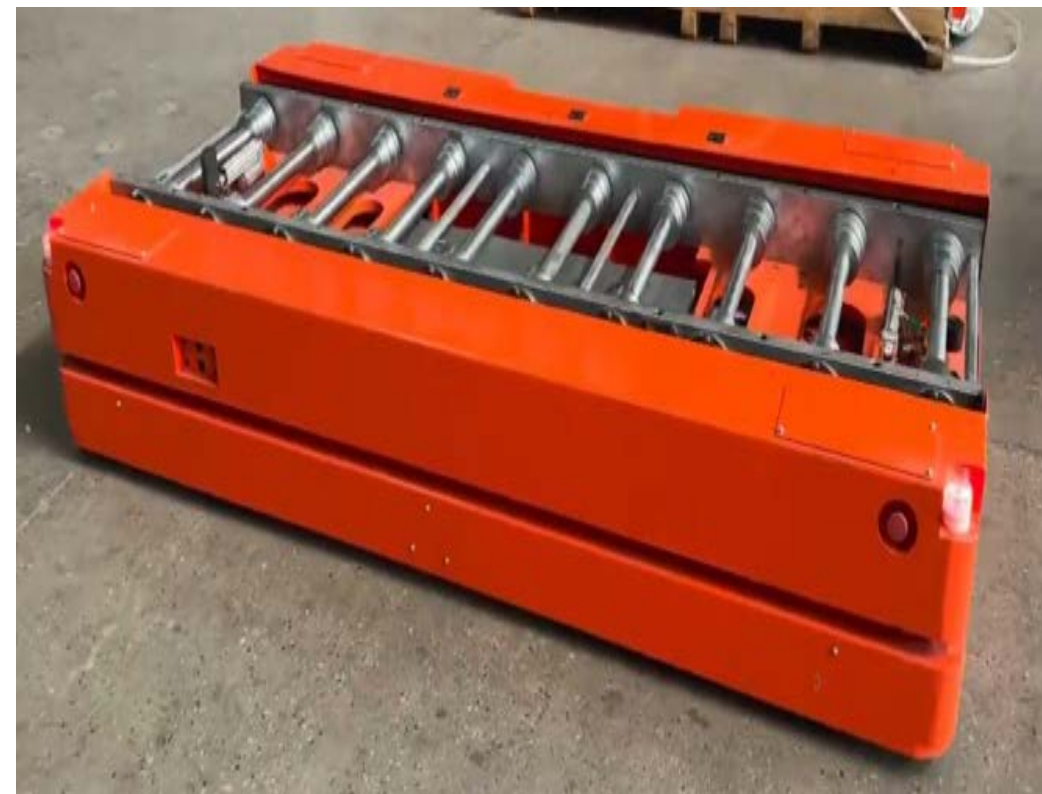
Engine Block AGV Transfer Equipment
