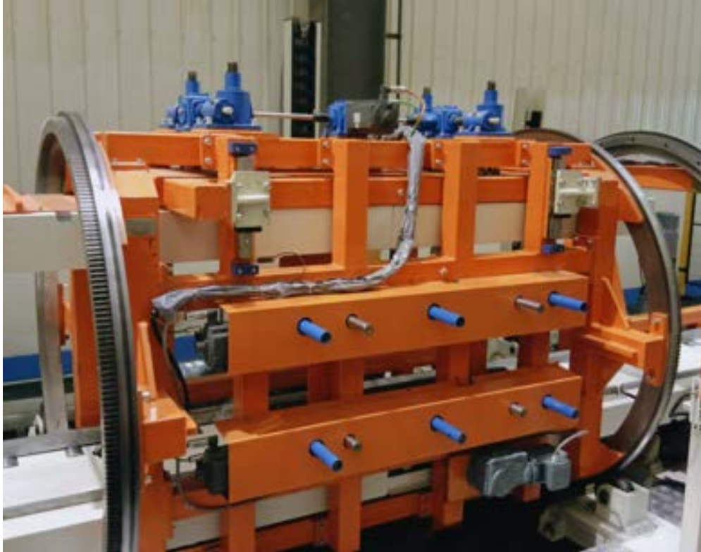
Automatic 180° Engine Block Turning Equipment
