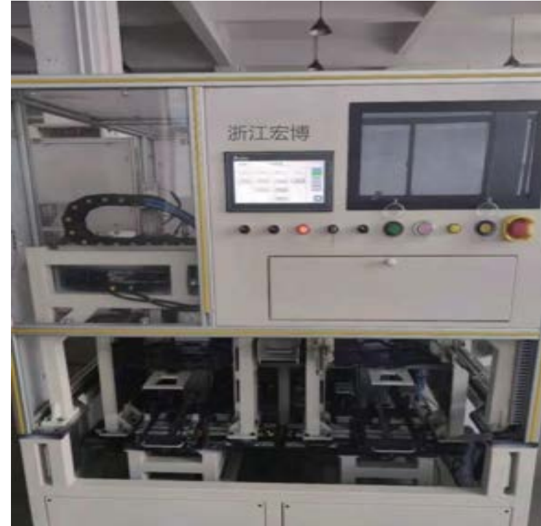
Battery Edge Voltage Testing Equipment
