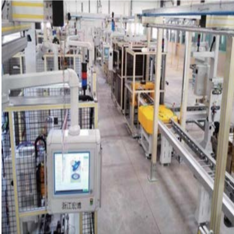
Engine Piston Pin Circlip and Propeller Shaft Sub-Assembly Line
